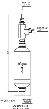
CS1-SS-CP (SS316 Condensates eparator with catch port)
